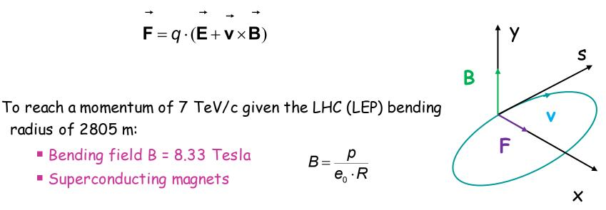
To collide two counter-rotating proton beams, the beams must be in separate vaccum chambers (in the bending sections) with opposite B field direction.
