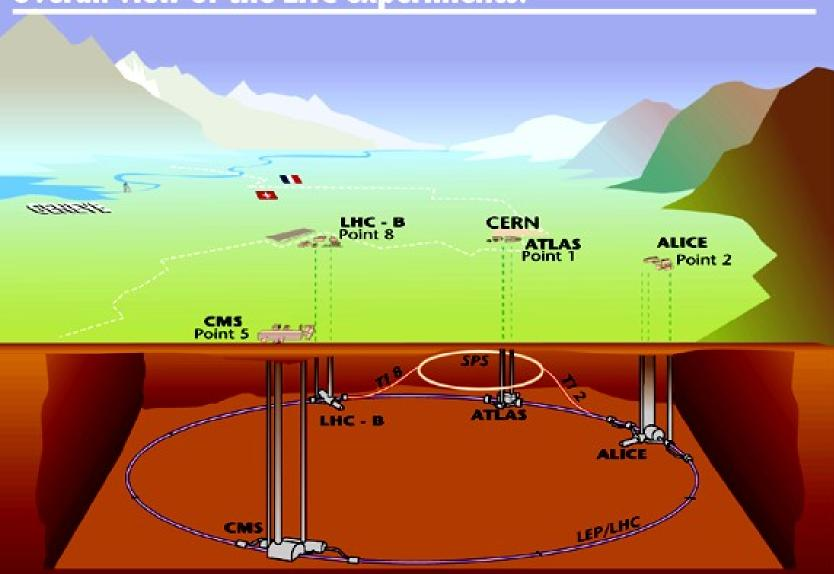
Tunnel circumference 26.7 km, tunnel diameter 3.8 m Depth : ~ 70-140 m - tunnel is inclined by ~ 1.4%
