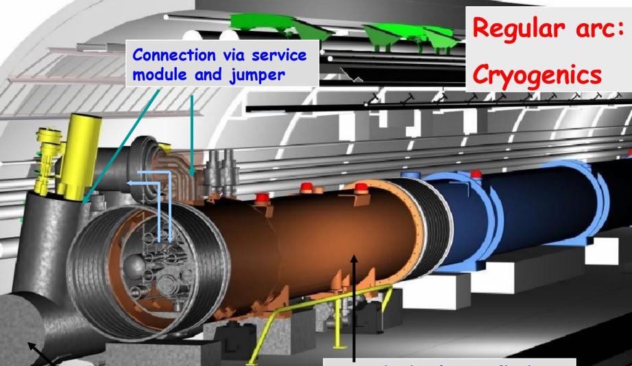
Supply and recovery of helium with 26 km long cryogenic distribution line Static bath of superfluid helium at 1.9 K in cooling loops of 110 m length
