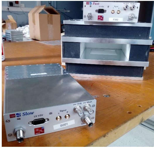
Chamber + Faraday Cage \sim 20 \times 15 \times 2 \text{ cm}^3
