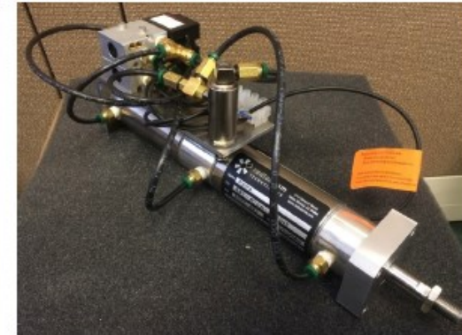
Dual Station Actuator retrofitted for new dual axis mask.
