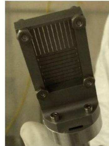
Dual Station Actuator retrofitted for new dual axis mask.
