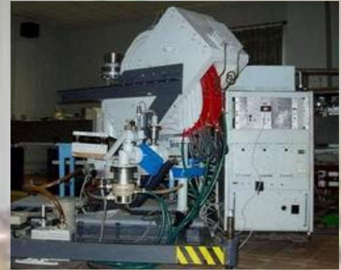
High-resolution magnetic spectrometer ( \Delta E/E = 3,2 \times 10^{-3} )
