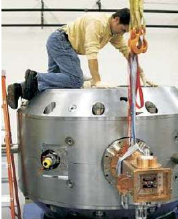
9 Tesla superconducting Synchro-cyclotron
