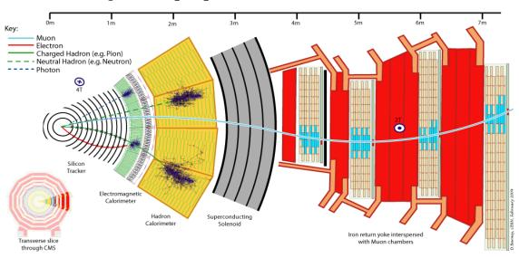
ECAL – crucial for  $H\to\gamma\gamma$  analysis, measures photons' energy. It consists of PbWO4 crystals For ttH production mode other subdetectors needed to reconstruct leptons and jets
