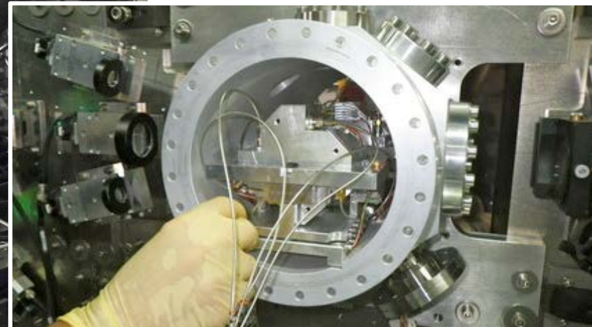
IP-BPM with mover in a vacuum chamber
