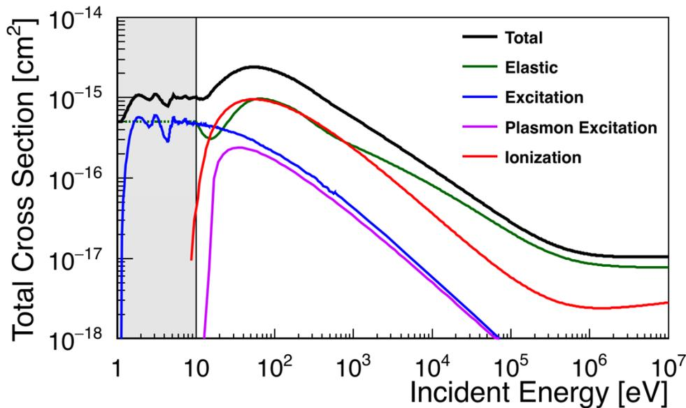
Integrated electron cross sections in gold. Bremsstrahlung is not shown. All particles with energy below 10 eV (shown in gray) are killed and their energy is dumped locally.
