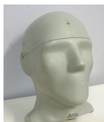
Figure 7.9. Typical phantom featuring a human skull, from X-ray absorption point of view.
