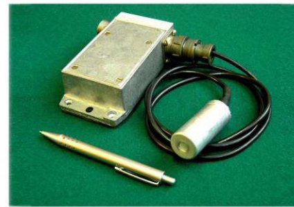
Detector module for X-ray dose rate control
