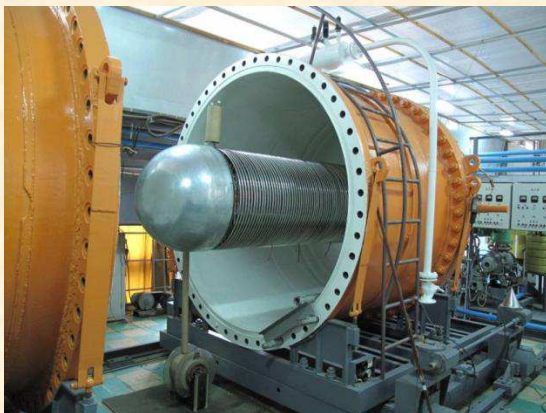
Accelerator for reactor radiation damage imitation
