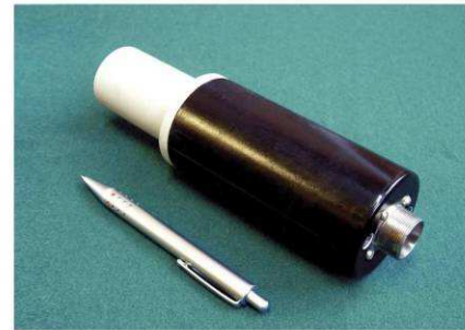
Wide-range \gamma -ray dose rate detector module
