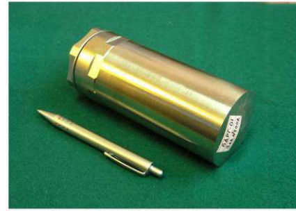
Emergency \gamma -ray detector module
