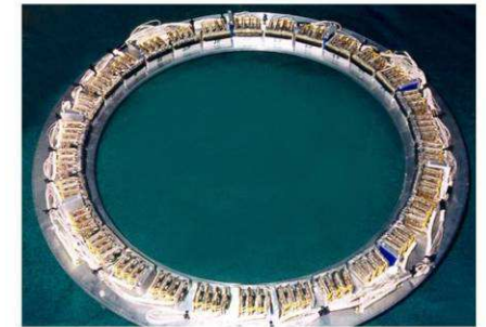
Circular matrix of 120 detectors with preamplifiers
