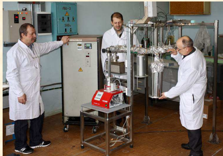
The complex pilot vacuum system for filling of the detector chamber with Xe
