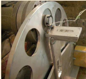
Test facility with CdZnTe detector ( 10 \times 10 \times 5 \text{ mm}^3 ) under electron beam (2.5 MeV).
