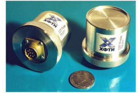
CdZnTe large-size spectrometry detectors ( \sim 1 \text{ cm}^3 )
