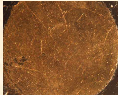
CdZnTe crystal (5x5x2 mm 3 ) with Pd contact deposited by restoring 0.4 %-solution of [Pd (NH 3 ) 4 ] Cl 2 .
