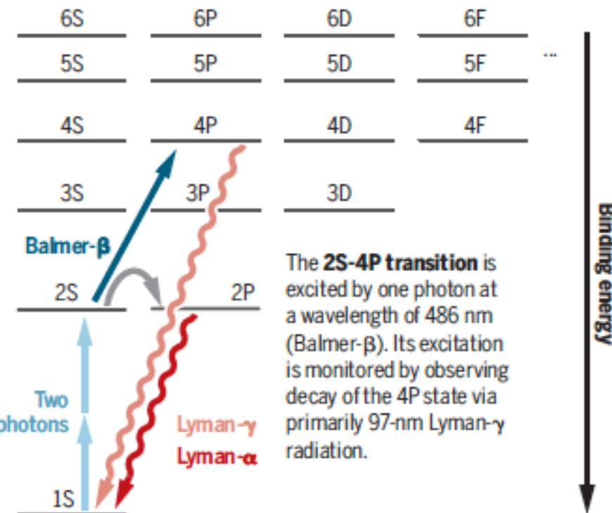
The **2S-4P transition** is excited by one photon at a wavelength of 486 nm (Balmer- $\beta$ ). Its excitation is monitored by observing decay of the 4P state via primarily 97-nm Lyman- $\gamma$  radiation.
