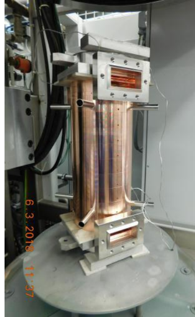
Prototype ready for Vacuum Brazing
