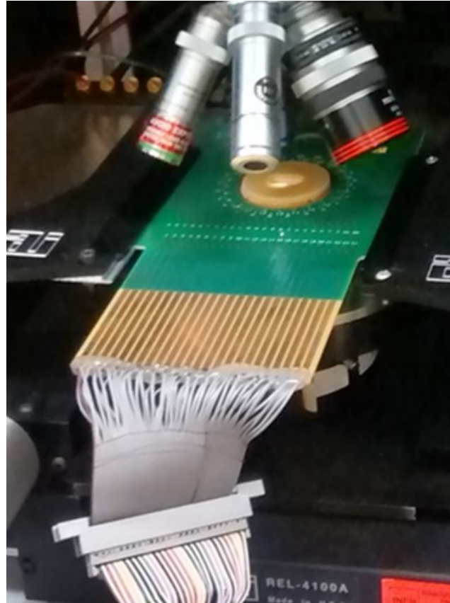
CUSTOM PROBE CARD FOR SIMULTANEOUS CONTACT TO ALLSTRIPS + GUARD RING
