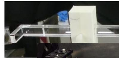
Quartz bars (2 channels, separated by 5 mm)
