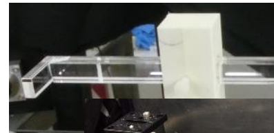
Quartz bars (2 channels, separated by 5 mm)
