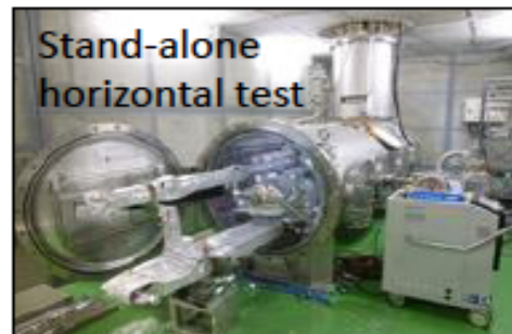
Module (including tuner, jacket)
