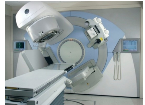
Clinical electron accelerator (X-rays ~6-25 MV)
