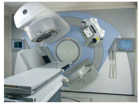
Clinical electron accelerator (X-rays ~6-25 MV)
