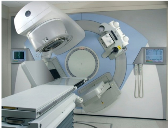
Standard clinical accelerator with embedded imaging systems
