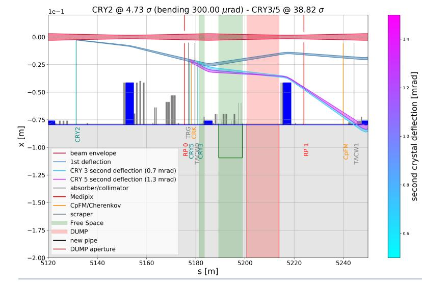
In LSS5, according to post-LS2 drawings, we could have **1 m** upstream the QF.51710. and **9 m** downstream
