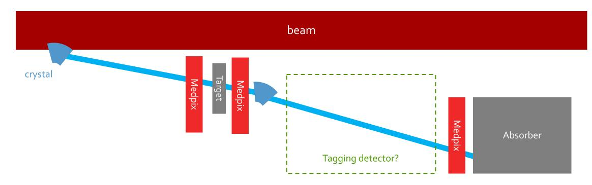
The schematic shows a conceptual layout of a double crystal setup for a particles tagging experiment. MediPixes can be used, but we might also have space for other detectors.
