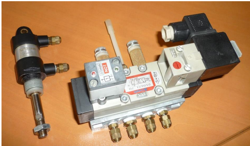
Actuator and electro-valve distributor.
