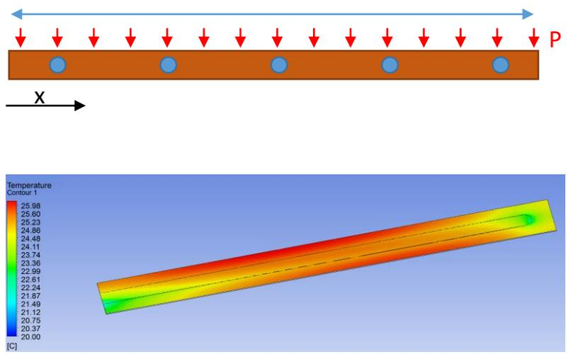
Thermal static CFD analysis thermal field example using Fluent with 100W extracted and water mass flow rate of 7g/s through 1,5mm ID pipe
