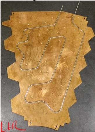
Pipe insertion on a cooling prototype
