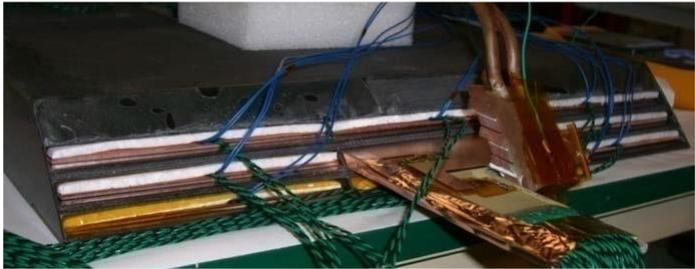
Passive cooling ramp set up test on a 3 layers prototype
