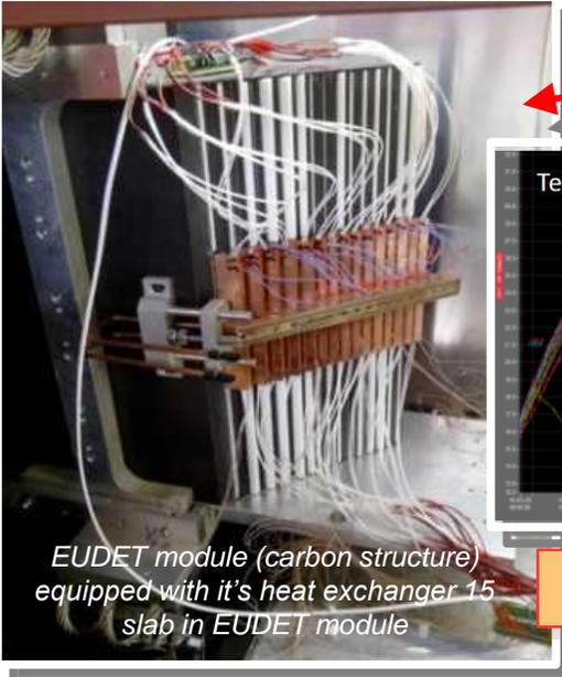
EUDET module (carbon structure) equipped with it's heat exchanger 15 slab in EUDET module
