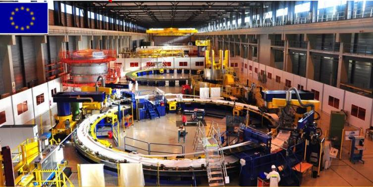
Four of ITER's six ring-shaped magnets (the poloidal field coils, 8 to 24 m in diameter) being manufactured by Europe in this 12,000 m<sup>2</sup> facility.
