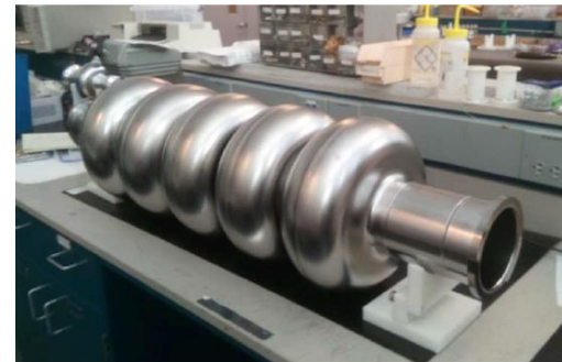
The first Nb 801.58 MHz 5-cell elliptical cavity fabricated at JLab [3].
