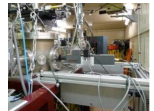
-120-1200°C irradiation in-situ \mu Raman
