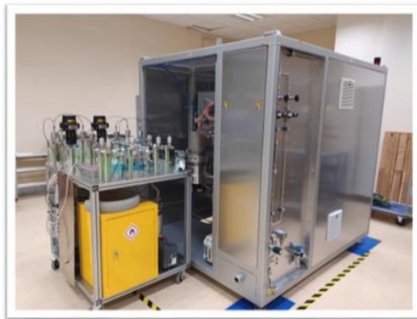
Picture of the new ALD system under construction
