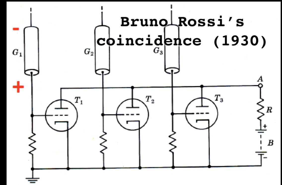
2 or more triodes coupled to G-M counters. When the grids were simultaneously driven to a negative potential by the coincident discharges of the 3 counters, a pulse appear at the plates.
