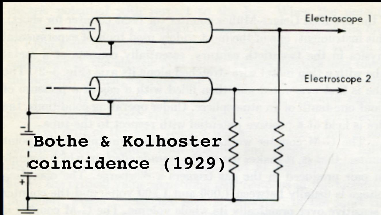
G-M counters (2 max) connected to electroscopes. When placed one above the other a small distance apart, often discharged simultaneously.
