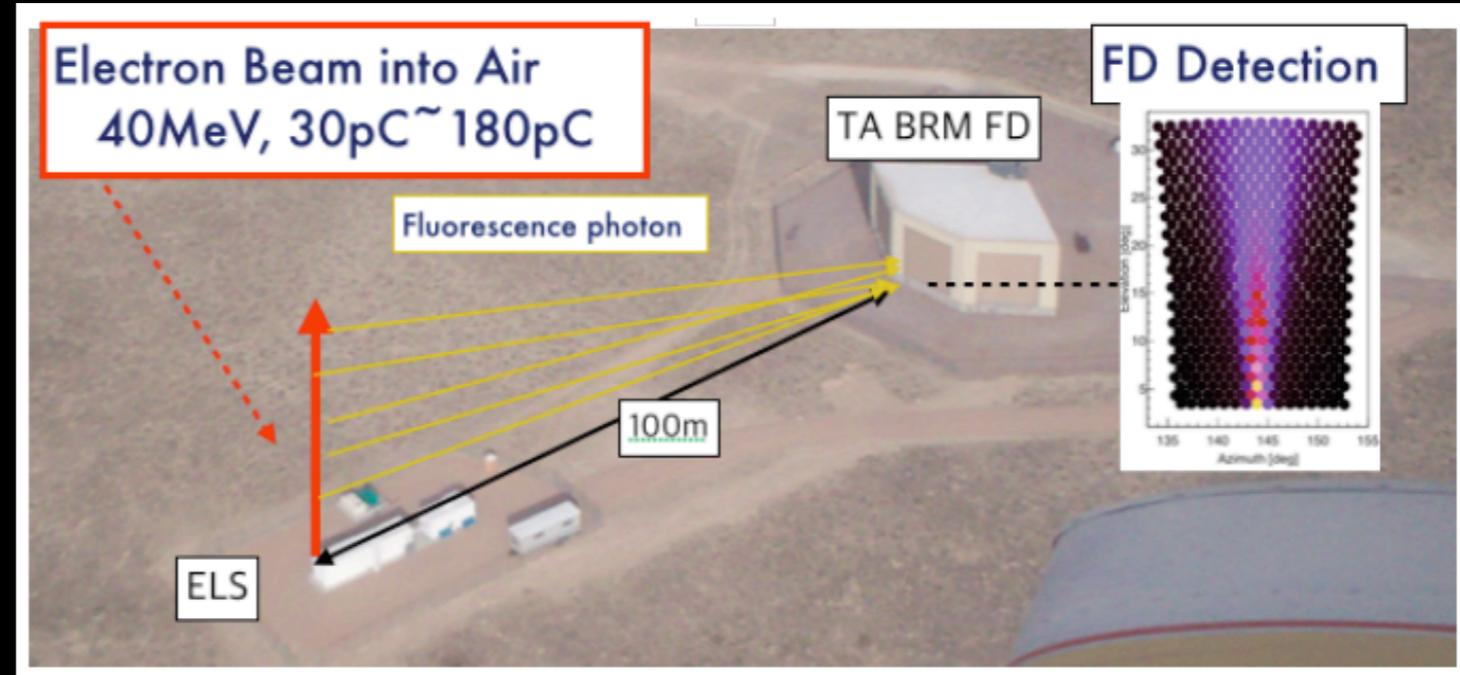
**THE ELECTRON LIGHT SOURCE IS AN ELECTRON LINEAR ACCELERATOR SERVING AS AN ABSOLUTE CALIBRATION. THE ELS FIRES A VERTICAL 40 MEV ELECTRON-BEAM OF DURATION 1 MS AT A REPETITION RATE OF 0.5 HZ.**
