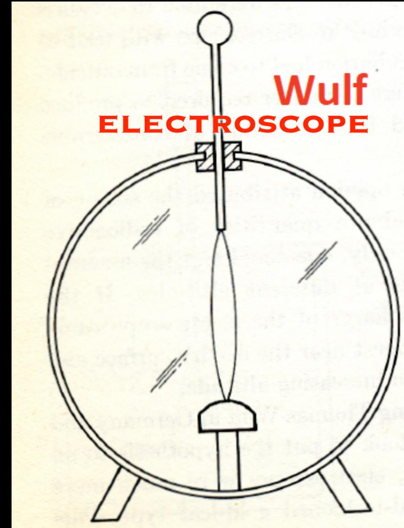
**First electroscopes developed at the end of the XVIII century.** When it is given an electric charge, the metal leaves (or wires) repel each other and stand apart. Radiation can ionise the air in the electroscope and allow the charge to leak away: leaves or wires slowly come back together.
