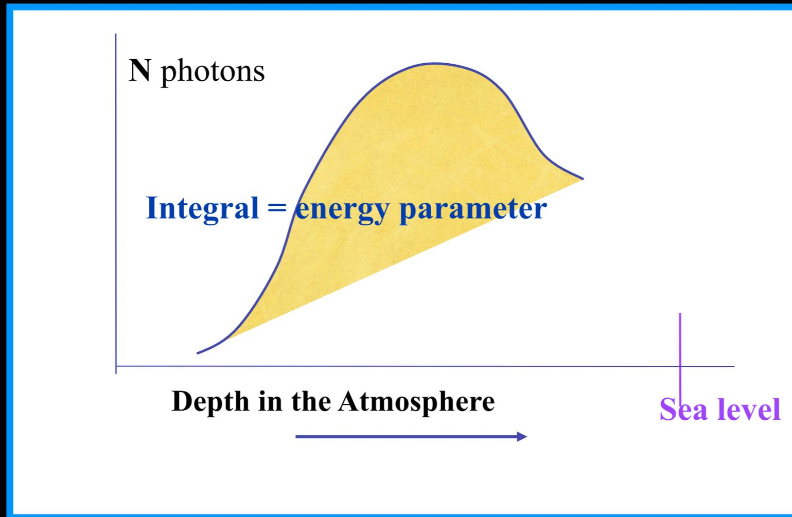
**Fluorescence detectors allow for a direct measurement of the shower energy deposited in atmosphere.**
