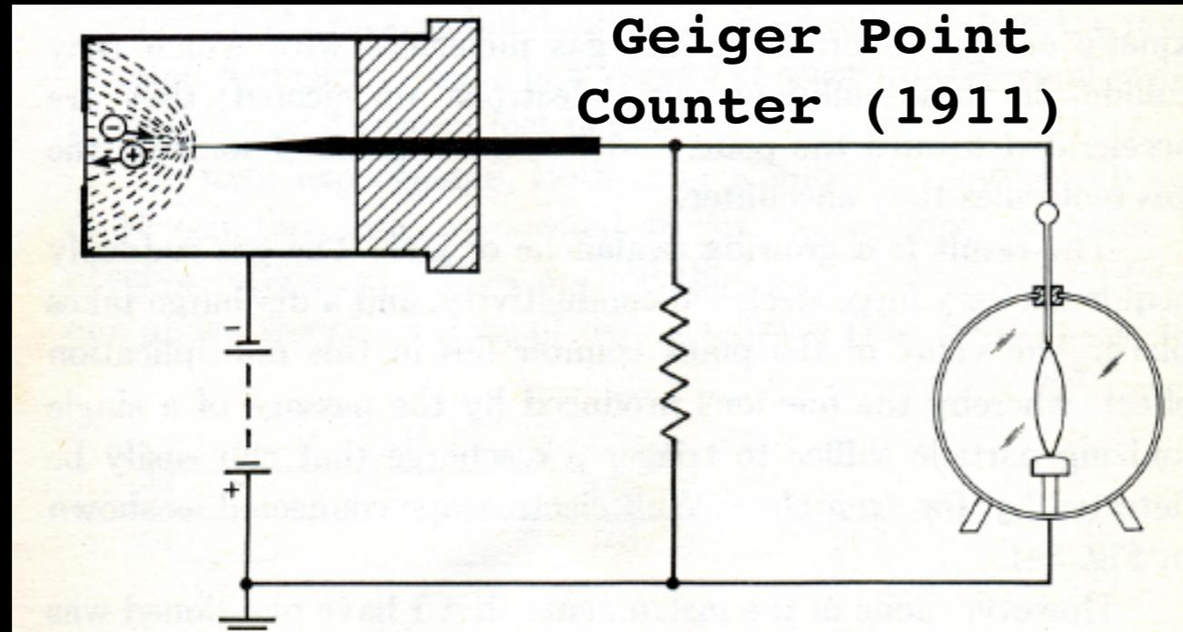
A thin point rod in a metal box filled with gas. A battery maintains the rod at positive potential with respect to the box. Particles penetrating in the box produce ionisation. Ions and electrons are accelerated: an avalanche creates a brief electrical current: the electroscope wires undergo a sudden deflection
