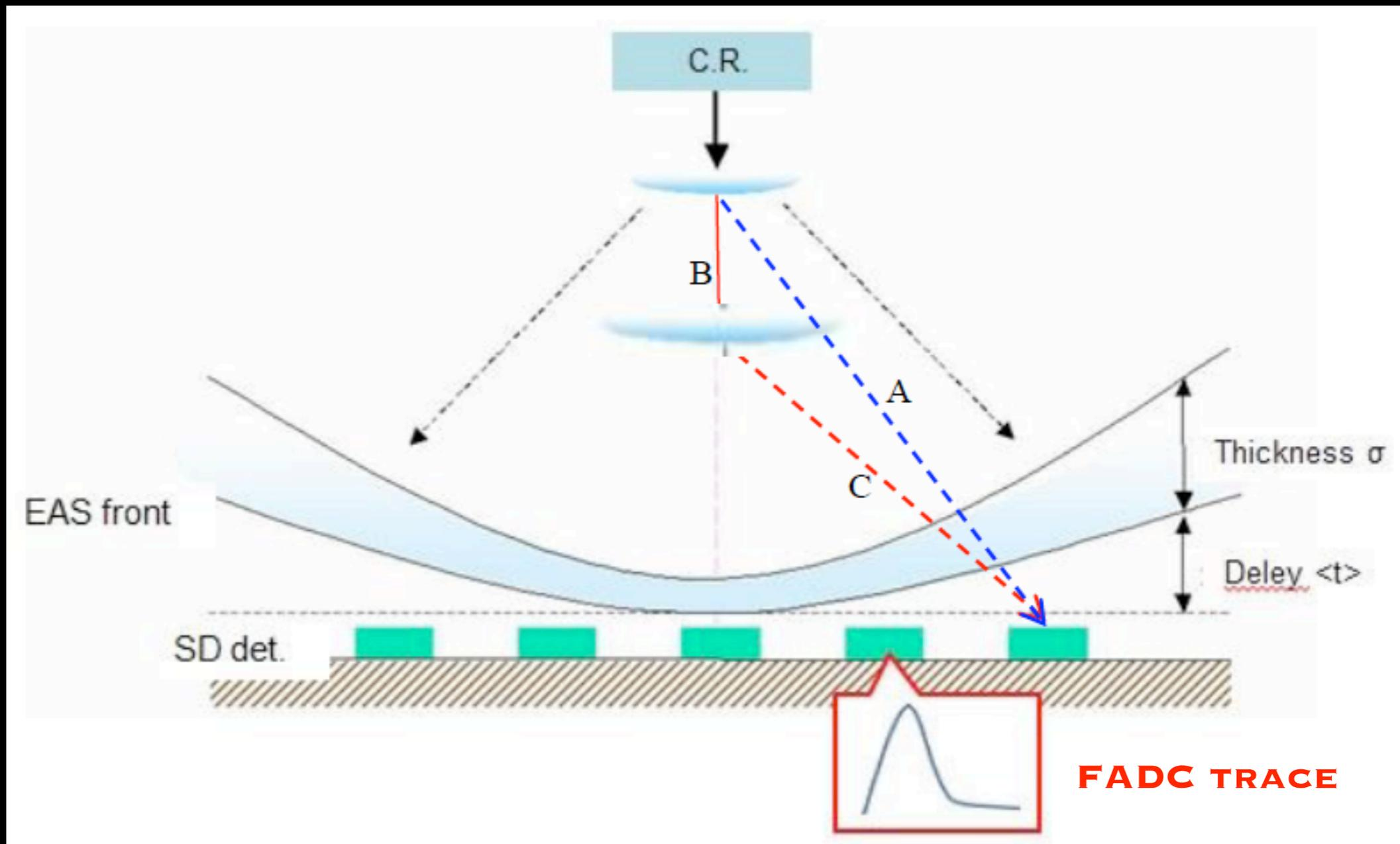
The PMTs signals are digitized by Fast Analog-to-Digital Converters (FADC), with a sampling time of 25 (20) ns
