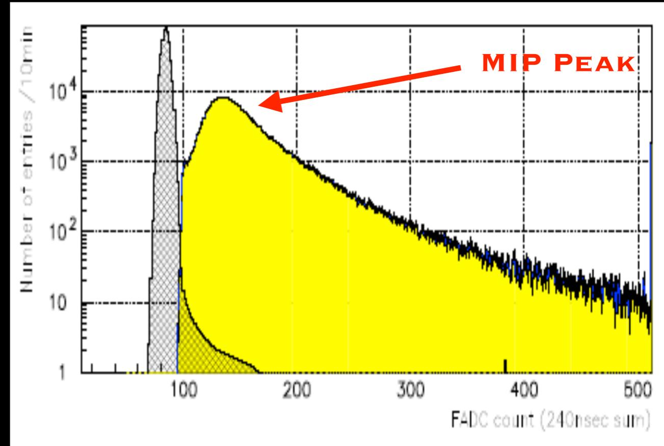
**CHARGE SPECTRUM OBTAINED (EVERY 10 MINUTES) WHEN A DETECTOR IS TRIGGERED (AT A LOW-THRESHOLD) BY THE COINCIDENCE AMONG THE PMTS (VEM = VERTICAL EQUIVALENT MUON; MIP = MINIMUM IONIZING PARTICLE)**
